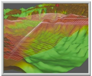
A terrain map with a portion of its mask shown. The red canopy represents the maximum height under which flying objects cannot be detected by the threats located on the terrain map
