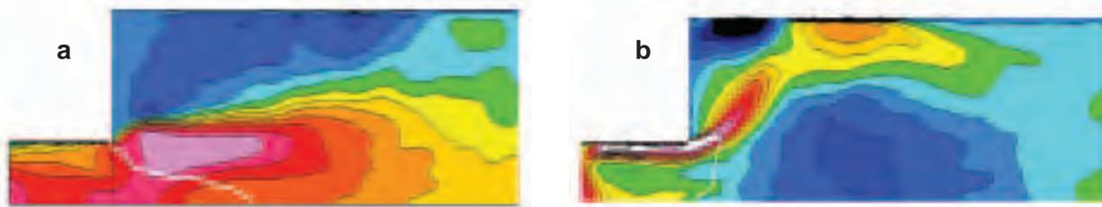
Figures 1a and b. Isocontours of axial velocity in the combustor for two different swirl numbers (left  $S = 0.56$ , right  $S = 1.12$ ). The colors red and green indicate left-to-right flow, whereas blue and black indicate reverse flow. As shown, increase in swirl creates a recirculating (reverse flow) bubble in the combustor that pushes the flame outward and also stabilizes the combustion.
