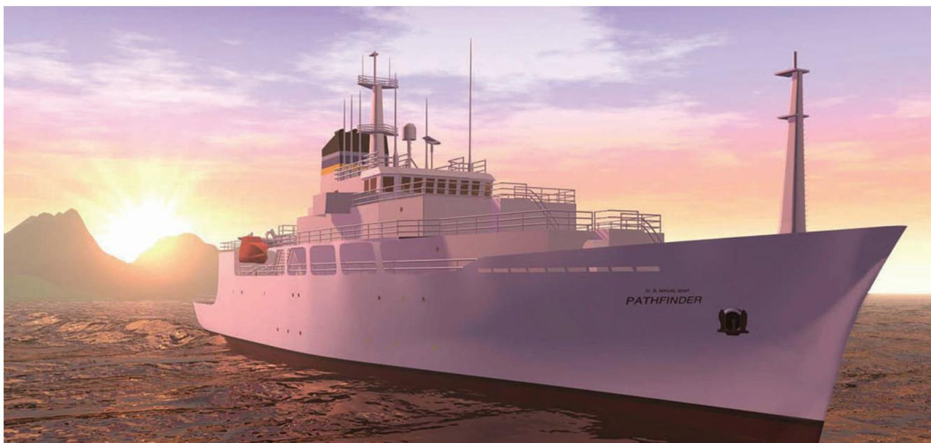
NAVOCEANO has technical control of six 329-foot-long, 5,000-ton T-AGS 60 class ships and one hydrographic ship designed to provide multipurpose oceanographic capabilities in coastal and deep-ocean areas. These include physical, chemical, and biological oceanography; multidiscipline environmental investigations; ocean engineering and marine acoustics; marine geology and geophysics; and bathymetric surveying.
