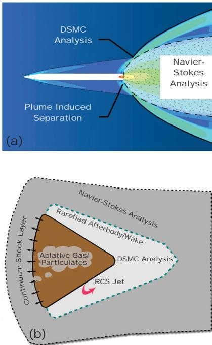
Figure 1. Examples of embedded continuum/rarefied flow fields.
