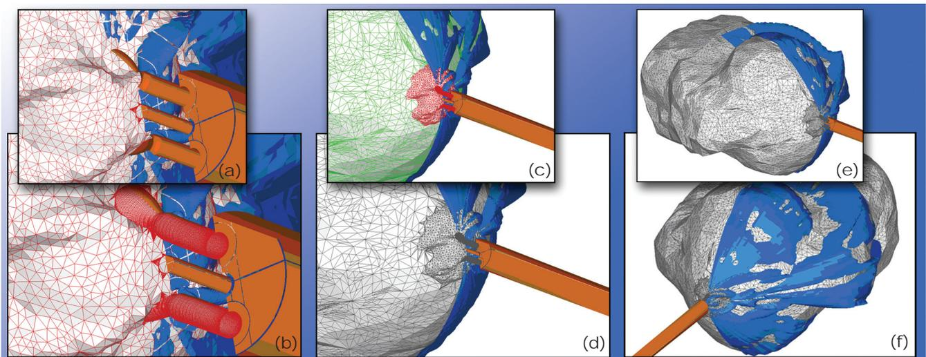
Figure 6. GTS Boolean operations on GDM generated surfaces.
