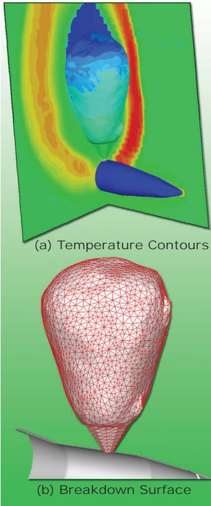
Figure 7. Hybrid solution for missile divert jet problem.
